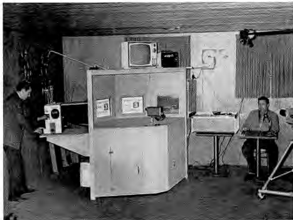
Local origination facilities at Gatlinburg, Tennessee, include 16mm sound-on-film, 2x2 slides, balops, flip cards, videotape, and local live. A time and weather system (not shown) completes the facilities. Studio manager Bill McMakin (left) prepares to insert a local live announcement to be delivered by general manager W. Marion Palmer.
