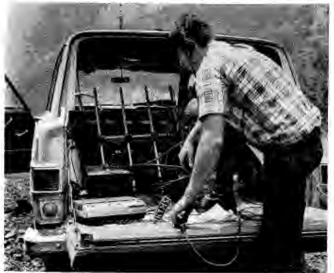
Some of KTMS's gear. In the foreground is a Sony portable tape recorder. Just behind this is a Moseley RPL-1 30-W Transmitter. The Jeep Wagoneer was both good transportation and mobile studio. The five element Scala yagi is used when high forward gain is required.
